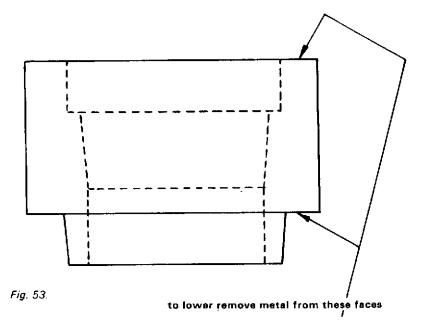
Again, if the ride height is excessive, adjustments can be made by machining one of the packing pieces.
