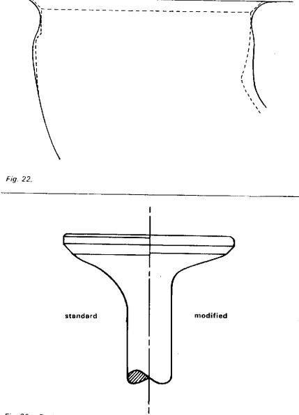
Fig. 23. Reshaped inlet valve.
