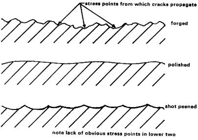
Fig. 41. Different types of surface finishes under magnification.
