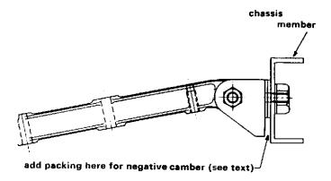
Fig. 55. Front suspension TR4A.
