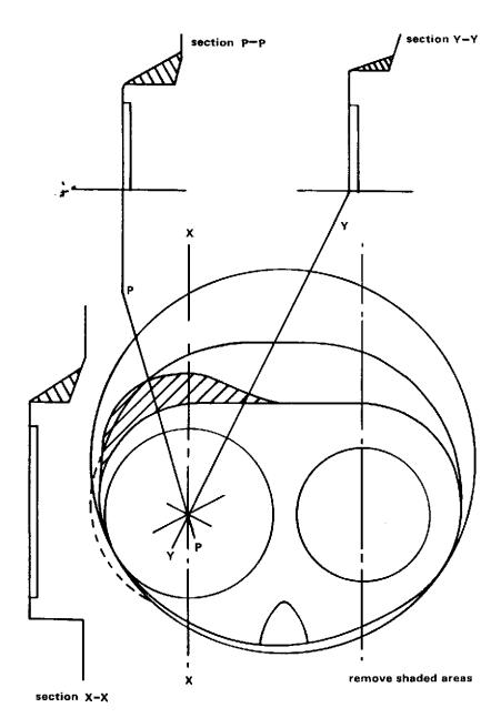
Fig. 36. Chamber modifications to TR4 and 4A.
