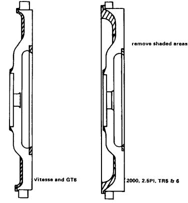
Fig. 46 Flywheel lightening.
