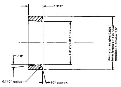
Fig. 33. Radiused valve seat insert.
