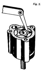
Measuring clearance between inner and outer rotors.
