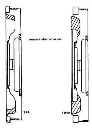
Fig. 46 Flywheel lightening.
