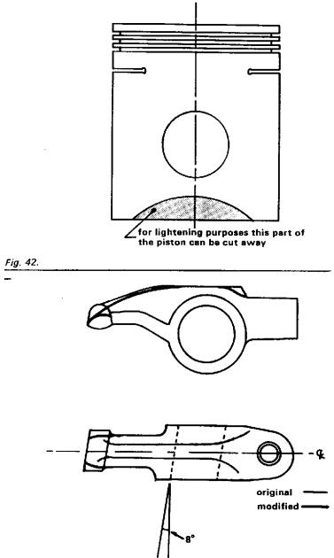
Fig. 43. Rocker lightening for 6 cylinder engines.
