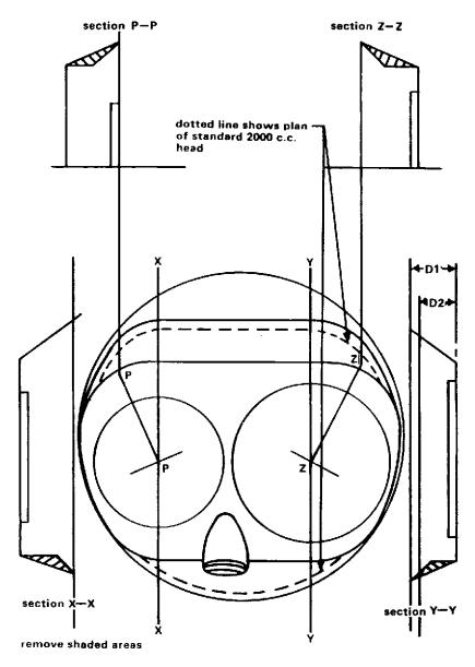
D1—standard chamber depth for 2.5 litre engines
