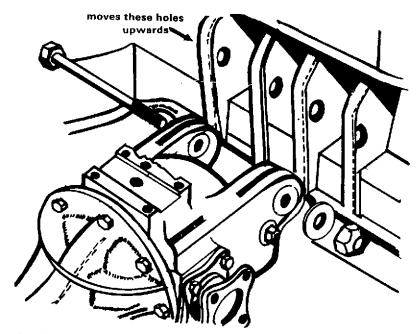
Fig. 60. Raising the differential on the Vitesses and GT6 Mk. 1 and 2s.
