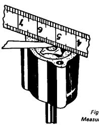
Fig. 7. Measuring rotor end-float.
