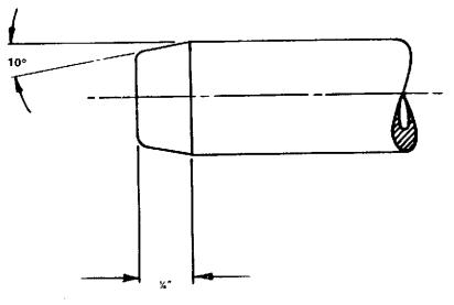
Fig. 32 Exhaust guide modification.
