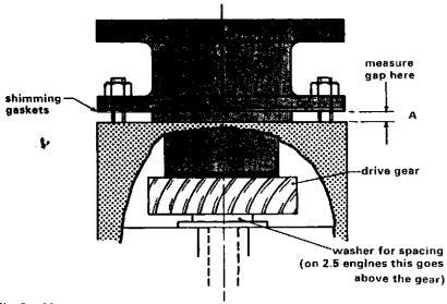
Fig. 3. Measure gap A and adjust with shimming gaskets until it is equal to the washer thickness +0.003 in. (the clearance). Having selected the correct shimming remove the washer and assemble parts as usual.
