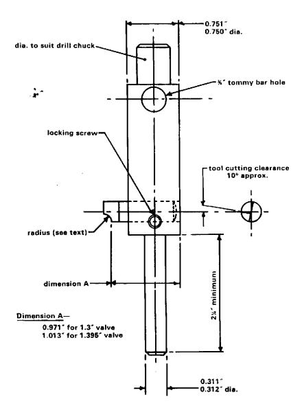
Fig. 21. Valve seat radiusing tool.
